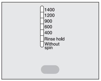
■ Press the "Spin" button repeatedly until the indicator light for the spin speed you want comes on.
